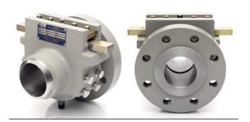
Canalta's Single Chamber Orifice Fitting incorporates the classic quick-change fitting design and adds HNBR O-ring seals for superior sealing capability. Built to meet or exceed ASME and ANSI specifications, as well as to comply with the latest editions of AGA 3 / API 14.3 and ISO 5167, these units are available in a wide variety of configurations, sizes and materials.
